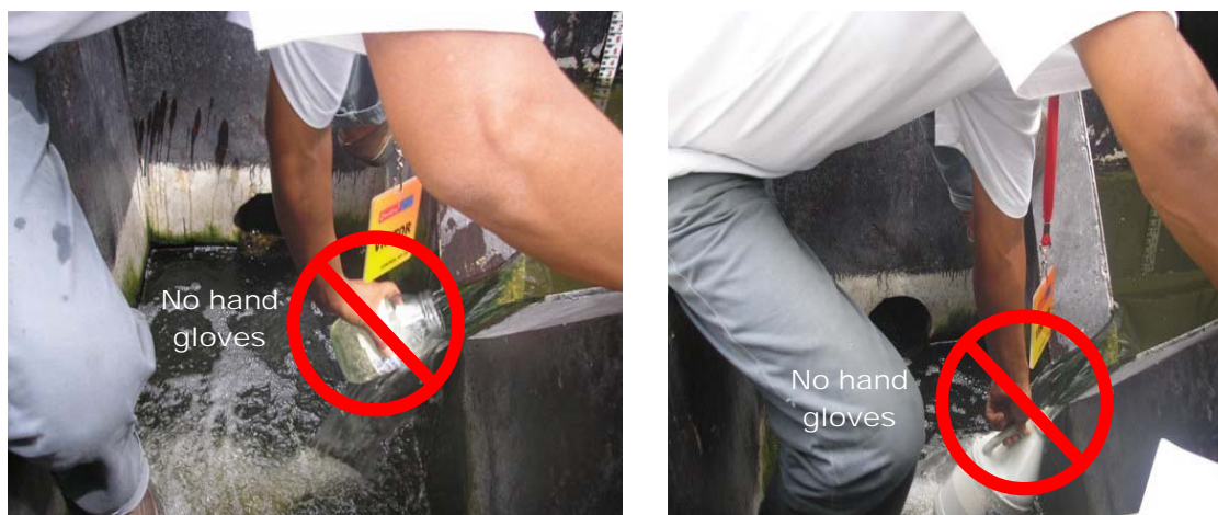
Figure 6.9 Effluent sample collection from a triangular weir of a restaurant by direct sampling with the sample container
