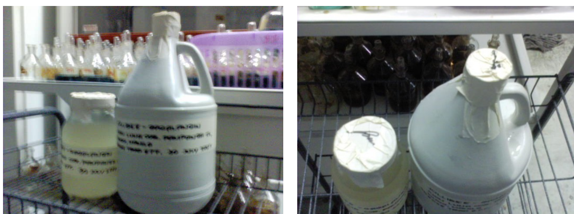
Figure 6.21 Labeled and Sealed Effluent Samples (Source: LLDA)
