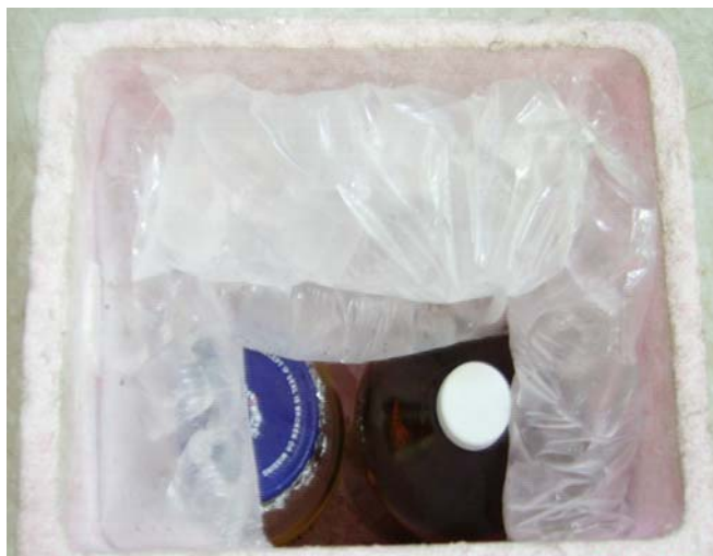
Figure 6.22 Samples Packed with ice in cooler
