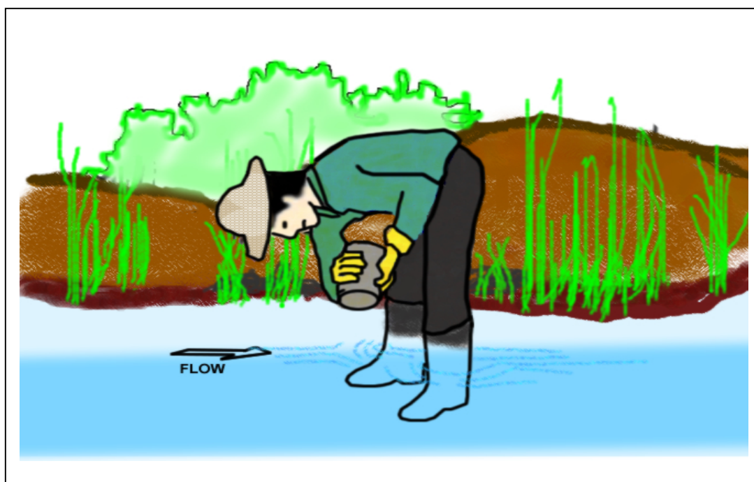
Fig. 4.3.1 (a) Proper Position in Taking Water Sample in Wadable Waters
