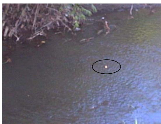
(d) Ball released from transect 1 floating towards transect 2. The time (in sec) it takes the ball to reach transect 2 is recorded.
